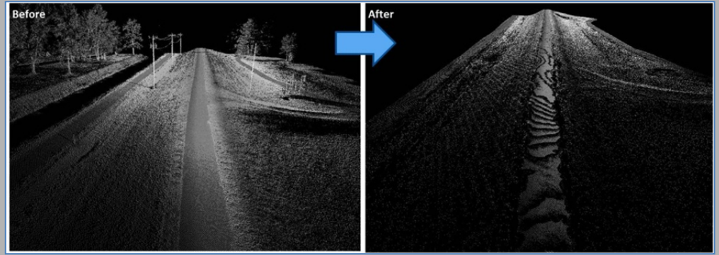
Figure 1: Un-cleaned Point Cloud on the Left, Cleaned "Bare Earth" Ground Points on the Right.
